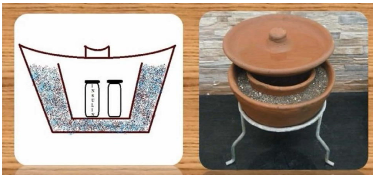
Fig 1. Double clay pot (wet sand between the two pots and water on the clay lid keep the interior of the pot cool) system for keeping insulin cool in the absence of a refrigerator ( photograph: courtesy Dr Archana Sarda, Aurangabad ).
